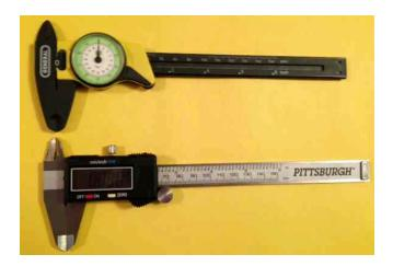
I've had, and frequently use, a General 6" Dial Caliper for a long time. Harbor Freight has digital calipers that measure both in millimeters and
