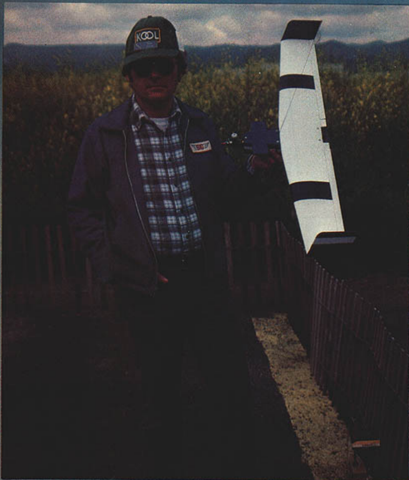
Dave Pastor displays his 1/2A RC cutie. He used a sliding servo tray for operating the strip elevons but notes that mechanical mixers will work just as well. Construction is super simple.
