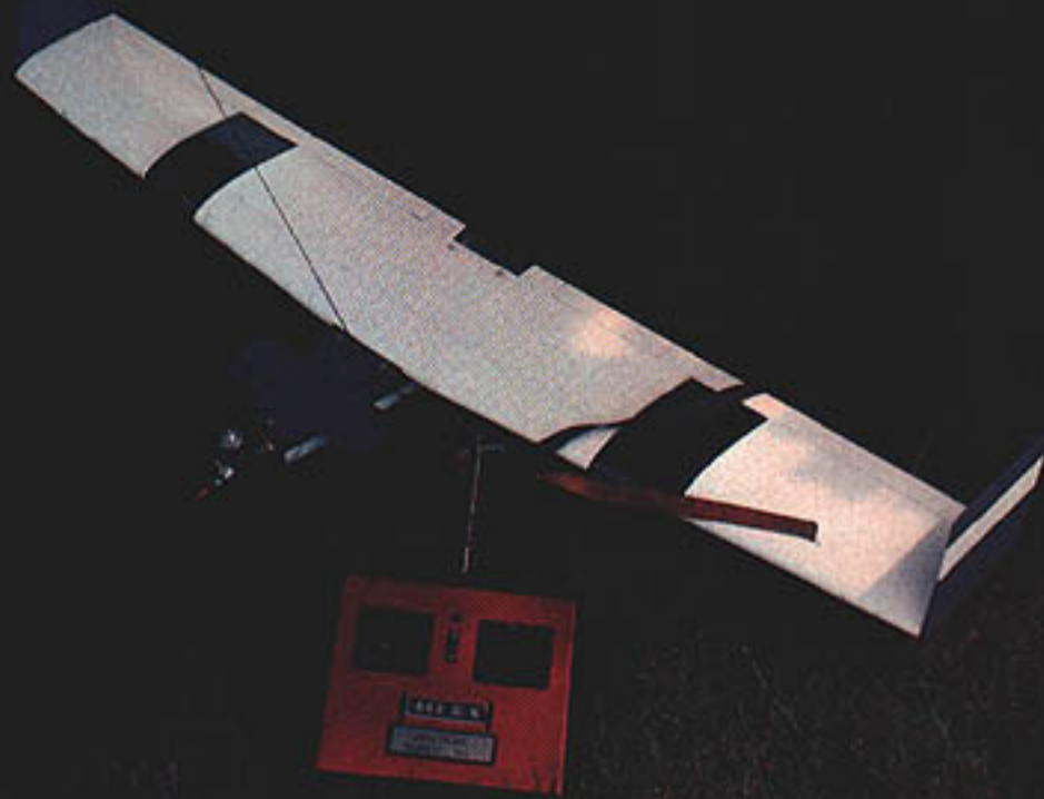
All you need for this one is a two-channel radio setup. It hand launches easily, and if you mount the prop horizontally as it begins to come up on compression, it will help save the prop on landings.
