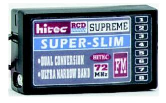
Supreme "Super Slim" 8 Channel FM Mini Receiver 8 Channel Dual Conversion Narrow Band 72 Mhz FM Receiver
