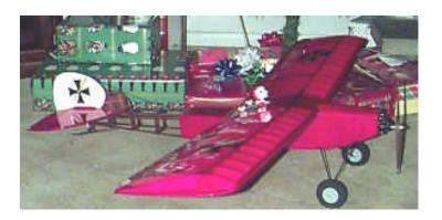
The aircraft is a just completed (12/21) TopFlite Elder 20, powered by a geared (Liesure 2.5:1) Astro Flight 035 and 7 cell 1700SCRC packs. All up weight with 1 ounce removable (velcroed) Snoopy Claus is 50 oz., first (and only, thus far) flight lasted 8 minutes, with power to spare.
