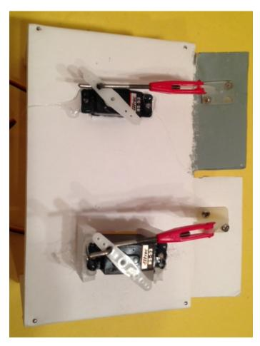
A second control horn, the Great Planes Large Nylon GPMQ3901, was attached to the other movable surface. Its outmost hole is approximately 1" above the top surface of the moveable surface. The servo, connected to the GP control horn, was raised so that the angle going from the servo arm connection to the control horn connection had approximately the same angle as the other servo arm connection to shorter control horn connection.
