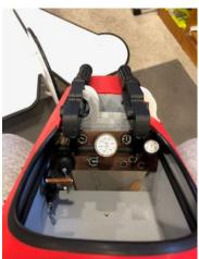
I added a pilot and seat and installed a new instrument panel including a tachometer, altimeter, fuel lever, fuel gauge, control stick, new ammo belts and magneto.
