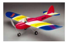
Specifications: Wingspan: 40 in (1015mm) Wing Area: 292.25 sq in (18.8dm2) RTF Weight w/270mAh NiCd: 11.4 oz (320g) Wing Loading w/270mAh NiCd: 5.6 oz/sq ft (17.1g/ dm2) Length: 26.1 in (665mm) Includes: 280 motor w/4:1 gear drive Requires: 3-4 channel radio w/mini receiver and 2 mini or micro servos, CS-10 ESC, 7-8 cell 270-550mAh battery pack, 9x6 Slo-Flyer prop
