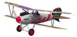
Specifications (Albatross D-V Bipe) Wingspan: 34 in (865mm) Wing Area: 360 sq in (23.2dm2) Weight: 12 oz (340g) Wing Loading: 4.8 oz/sq ft (14.5g/dm2) Length: 37 in (940mm)
