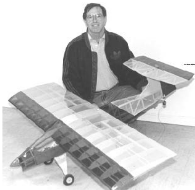
Tom Hunt, chief designer of MODELAIR-TECH, with his new ultra-large sport electric model called the MEGAWATT - 7.5 pounds total weight with an H-1000 belt drive and an inexpensive DeWalt drill motor. Full kit to be available in 1996.
