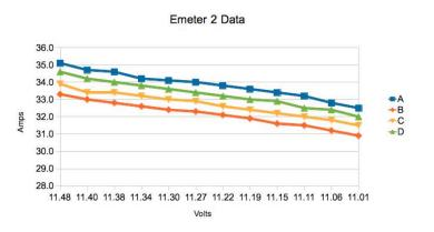
The graph above shows the amp draw data for two APC 13x6.5E thin electric props and two APC 13x8E thin electric props as recorded by an Emeter 2 at similar voltages. The props are labeled A, B, C, and D for the quiz. Use the lines below to indicate which prop you believe is represented by each line in the graph. Remember there are two of each prop. A: \_\_\_\_\_\_B: \_\_\_\_\_ C. \_\_\_\_\_D:
