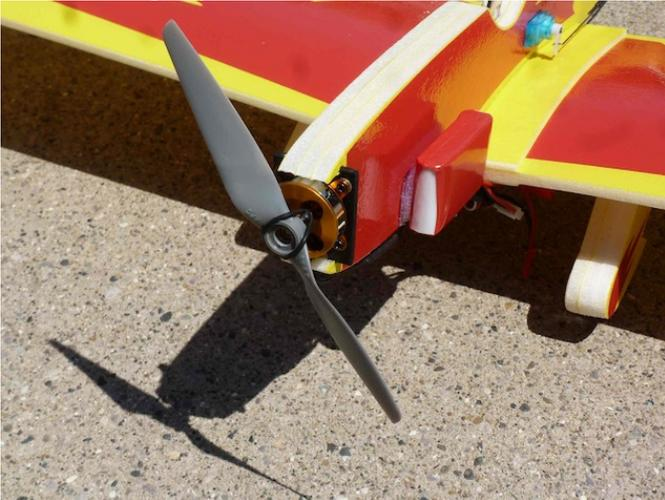
With the motor mounted, the ESC can be double sided foam taped to the bottom of the fuselage.
