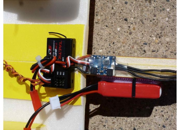
The receiver is held to the bottom of the wing with double sided tape.
