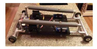
Hank Wildman shared one of the most unique things I've seen in my long RC career. He created a launch vehicle for his new Twister with a 70mm fan. The launch vehicle is made mostly of PVC pipe and parts from the RC car world. The vehicle is powered by two old motors from past Twisters. The vehicle is driven and steered by another person, as the plane, flown by the pilot, flies off of it. It took a lot of unsuccessful tries to get it right, but it IS working now. I'd love to see it in action!
