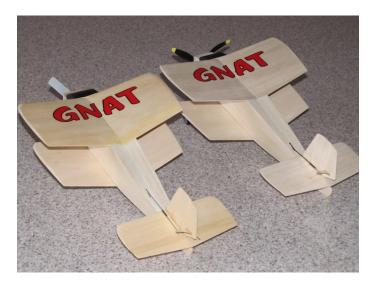
Trying to save some weight I built another (aircraft on the right) with better wood, a Park Zone brick and a Park Zone geared motor from their Trojan, three bladed prop and a single 220mAh Li-Po.
