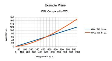
If the 250 sq.in. plane had a wing area loading of 24.42 oz./sq.ft., like the 1000 sq.in. plane, it would weigh 42.4 oz. Flying a 250 sq.in. model at this weight is challenging.
