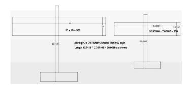
For the smaller model, with a 250 sq.in. wing, to have similar flight characteristics, providing it is designed properly to fly at the reduced scale, it would have to have the same WCL of 9.27 as the larger model. It should weigh,  $(250/144)^{1.5} * 9.27$ = 21.2 oz. ready to fly (RTF). The wing area loading of the 250 sq.in. would be, 21.2 oz. / (250 sq.in. / 144 sq.in.) = 11.65 oz./sq.ft. That is quite different from the 500 sq.in. model's wing area loading of 17.28 oz./sq.ft.
