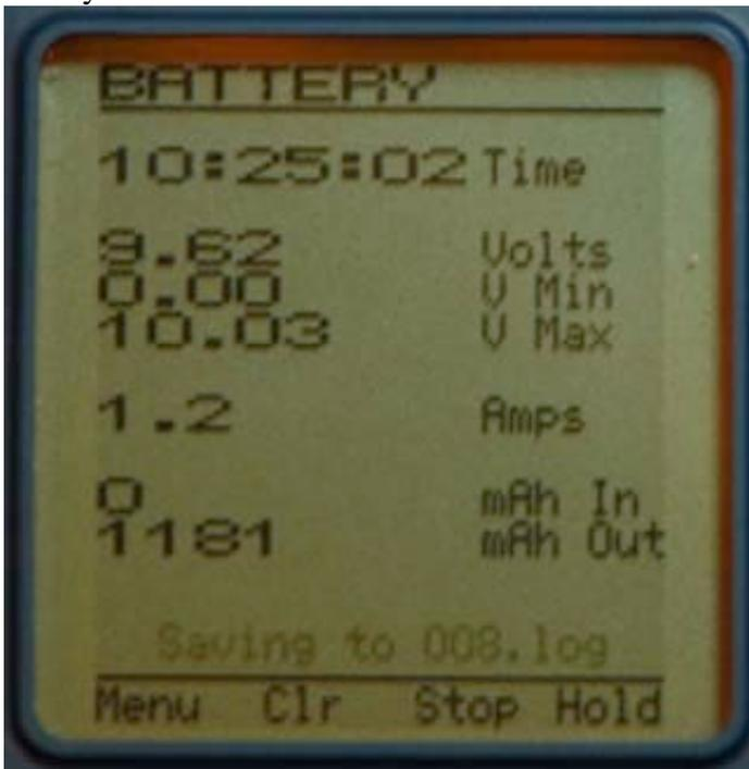
The Emeter II screen shows that at 10:25:02 I had discharged 1181mAh. The battery was at 9.62v and the discharge had started when the pack was at 10.03v. My AF 109 on discharge is drawing 1.2 Amps. It also shows that I'm logging this part of the discharge to 008.log. I can stop the logging process by a press of the C button under the word Stop.
