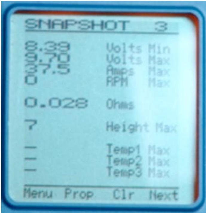
0.028 Ohms divided by three equals 0.0093 ohms per cell, and matches what was displayed on the CellPro 10S.
