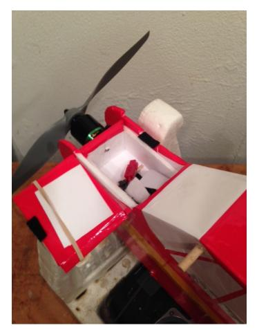
A new piece of DTFB, that I call the battery protector, was cut to fit and glued behind the firewall. It fits behind the firewall and has a hole for the motor shaft.
