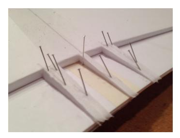
There is a gap between the "rear spar" of the wing and its trailing edge. I cut 5 triangles from
