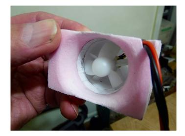
almost 90 sq.in. yet weighs only 2.1oz with the 2 cell 250mAh LiPo. Static thrust is 1.9 oz.
