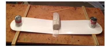
A brick was also used to weight the center section as I lifted both wing panels equally to encourage the dihedral bend.
