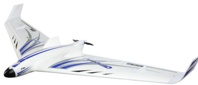
HH E-Flite Opterra 2M Flying Wing BNF Basic with AS3X 1033 sq. in. / 144 = 7.17 sq. ft. 69 oz. / 7.17 sq. ft. = 9.6 oz./sq. ft. Stall Speed = 11.5 mph
