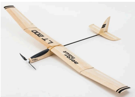
Aero-naut LT 200 Flex 468 sq. in. / 144 = 3.25 sq. ft. 30 oz. / 3.25 = 9.23 oz./sq. ft. Stall Speed = 11.2 mph
