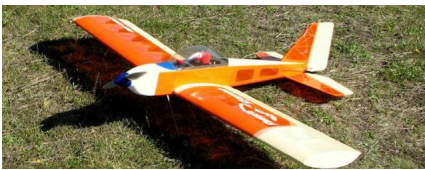
Mountain Models Switchback Sr. 600 sq. in. / 144 = 4.17 sq. ft. 38.3 oz. / 4.17 = 9.18 oz./sq. ft. Stall Speed = 11.2 mph
