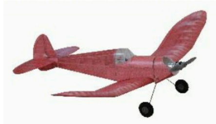
BMJR Panther 299 sq. in. / 144 = 2.08 sq. ft. 19.8 oz. / 2.08 = 9.52 oz./sq. ft. Stall Speed = 11.4 mph
