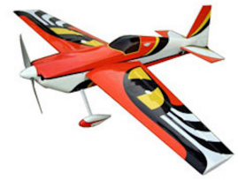
StevensAero Edge 540 Pattern 3D Acrobat 440 sq. in. / 144 = 3.06 sq. ft. 30 oz. / 3.06 sq. ft. = 9.80 oz. / sq. ft. Stall Speed = 11.6 mph
