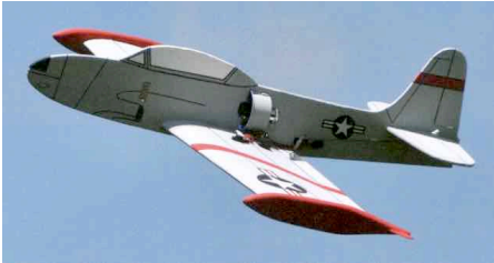
Lockheed T-33 (foam-plans) 400 sq. in. / 144 = 2.78 sq. ft. 25 oz. / 2.78 = 8.99 oz./sq. ft. Stall Speed = 11.1 mph
