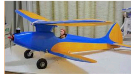
Retro RC Chicken Hawk 236 sq. in. / 144 = 1.64 sq. ft. 16 oz. / 1.64 = 9.76 oz./sq. ft. Stall Speed = 11.6 mph
