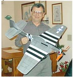
Rick also shared his Freedom 3D. He said that it is perfect for electric because it is built very light. Unfortunately it may be too light in the landing gear area, so he reinforced that area. He's using a Hitec receiver with HS-85 and HS-81 servos. The motor is a Mega 22/2-/3 with a 5:1 MEC gearbox. The pack is a 10-cell GP-3000. It weighs 63 oz. ready to fly, has a 48-inch span and a wing area of 675 sq.in. It flight great. It hovers well and pulls straight up out of the hover with authority.
