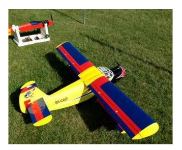
The photo shows the new red bands paralleling the top center section. The bands cover the open Maxlok key tab surgery and some balsa repairs on the top sheeting.
