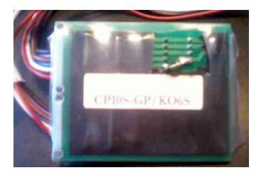
I wanted to use the solder wire as a jumper but without precise heat control and a steady hand it simply melts. I had to make a jumper out of an old servo wire.
