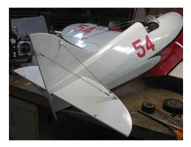
vertical stabilizer bracing/rigging. The model had no provisions for upper wing rigging and tail rigging, which I dutifully added. The black striping on the model is much too wide, but I think I'll leave it that alone. I'll be using the 15x8 APC prop like Greg Gimlick used, a Cobra Scorpion 3525/12 motor and a 60 amp Scorpion speed control, with built-in switch mode BEC, and 4S 4500mAh LiPos.
