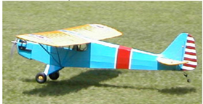
84" span, 8lb 20z, 20 x 2000mA NiMH cells and a MaxCim 13Y on 3.3:1 and a 15x8 APC-E - flies just like a Cub! The photo attached is her about to touch down - she's still a tad nose heavy, hence the near full up elevator as I flair to land. Superb kit, really simple conversion - I hardly did anything, beyond fitting a funny shaped 'engine' under the cowl and a larger 'gas tank' up front.
