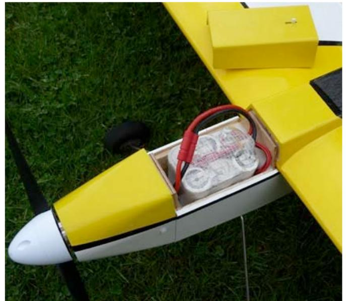
The motor is a Turnigy SK4250-650, powered by a 6S1P A123 pack, which produces 575 Watts @ WOT with a 12 x 6 EMP prop. (9660 rpm @ 17.63V and 32.6A). It gives me about 5>6 minutes of 'spirited' flying.
