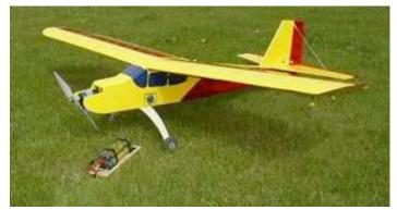
First is my conversion of a Sig LT-40. The fuse was replaced with a balsa structure of the same design and the original formers were used. I enlarged the front hatch to accept a battery tray, which holds up to 18 cells.
