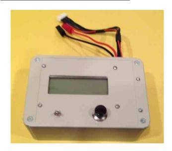
Next he showed a Battery IR meter designed by Denny Volrath. It is NOT a commercially available unit and must be assembled from components listed in the build thread on RC Groups.
