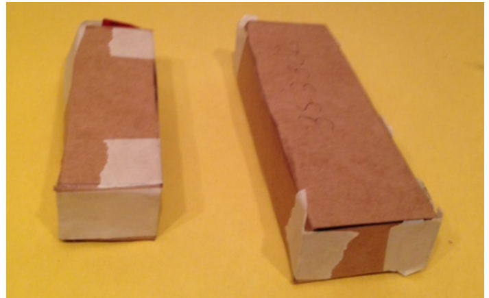
Dummy LiPo Batteries, Constructed from Cardboard for the Falcon 56 MK II
