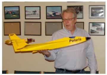
It has a wingspan of 29" and is 38.4" long. With a wing area of 343 sq.in. and flying weight of 9.1 oz. it has a wing loading of 3.82 oz./sq.ft. and wing cube loading of 2.48 oz./cu.ft. It is outfitted with a Spektrum AR6100 receiver, 3 Spektrum DSP75 servos, CC Phoenix 35 ESC and a Hacker A20-12XL outrunner. It uses an APC 7x4SF prop and a3S 2070mAh Li-Poly battery.
