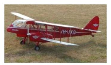
http://mysite.verizon.net/milkyway99/id3.html A biplane twin like the de Havilland DH-84 Dragon-2 or the DH-89 Rapide are good choices. The biplane configuration lowers the WCL. With no retracts the weight is kept down and construction kept simple.
