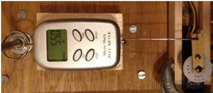
The idea for this servo torque tester came from an RC Groups thread named "Servo Torque Tester".
