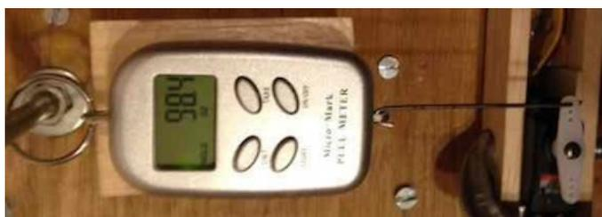
A standard servo arm was attached providing a 9/16" or 0.5625" lever.
