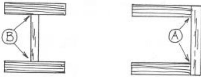
glue is not very strong in shear. There is not a lot of gluing surface. A good shear web in-between the spars is stronger, because the joint at "B" is not in shear and the glue is just there to hold it in place - not really much load on it.
