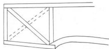
If you think about it, as you come into land, the motor wants to continue down and this diagonal, in compression, prevents the bay from parallelogramming. The triangle is doing its job. You can also put one going the other way.
