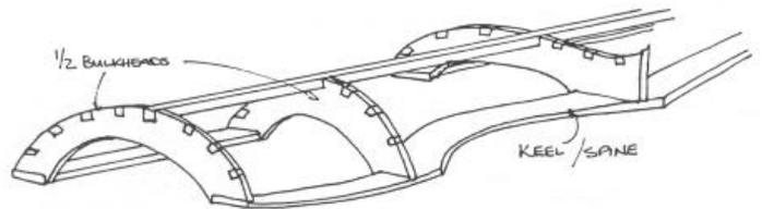
Essentially you are building a complete half of the fuselage. After finishing it, unpin it from the board, add the remaining bulkheads and the remaining stringers. If everything was done properly, it should end up straight. This is building on the half shell. The Mew Gull and the Spitfire were done this way.
