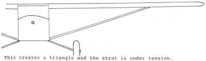
This creates a triangle and the strut is under tension.
