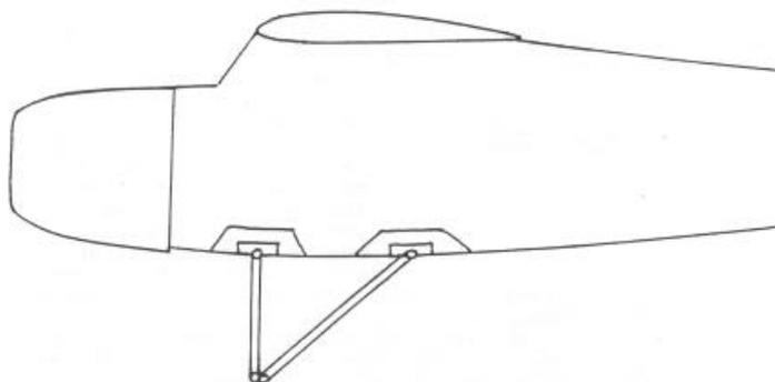
Like the trunnion block gear, this type also flexes out. Smaller diameter wire can be used than with the torsion bar landing gear of the wing. Use 1/8", 5/32", or 3/16" (for big planes), in wing torsion bar gear while 3/32" or 1/8" will work with this type of fuselage gear.
