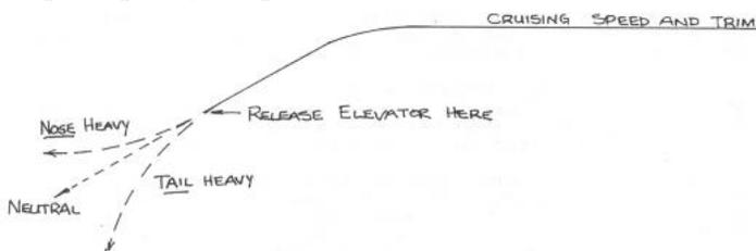
If the stick is released, and the airplane tries to do a half loop, the airplane is very **NOSE HEAVY**. When the airplane picks up speed, the negative incidence, (or slight up elevator trim), acts like up elevator and will try to make the plane loop. (The increased speed makes the trim have more effect.) As the CG is moved back, there is less of a downward load on the tail, so speed has little or no effect.
