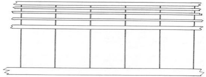
If you touch one wing tip on landing, the whole wing panel will try to parallelogram.
