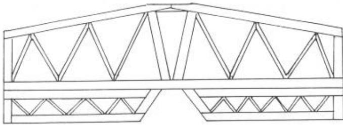
If you're worried about having the lumps showing through the covering, you can use a combination of these two. Put in the needed ribs and put in 1/8" x 1/16" diagonals that don't touch the covering.
