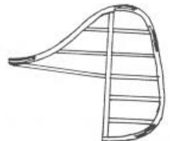
laminations, wrap it around the ply or foamboard form and tape it in place. Let it dry, take the tape off, pin it down and fill in inner structures. You can use 1/32" strip for the really small airplanes. It is very strong, like eggs and circles. It weighs virtually nothing.
