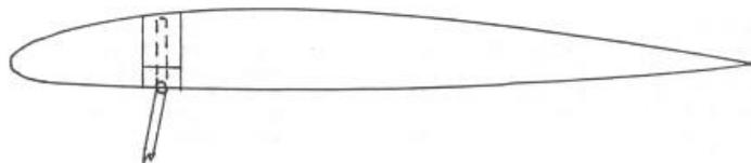
If you want to do a trunnion block set up use 1/32" ply laminated to the rib and notched to the spars. The
