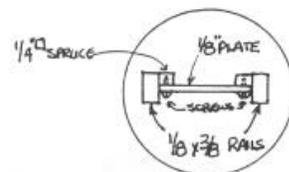
When the correct balance is achieved the plate can be secured with screws.
