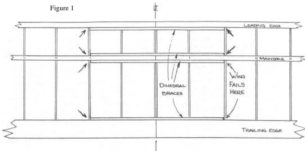
shear webs BETWEEN the spars. An "I" beam is much, much stronger. If you think about a wing, as the tip flexes up, the two spars appear to slide in opposite directions. The shear webs prevent this.
