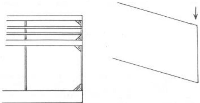
With the grain parallel to either side, it's not doing any good. As soon as there is any strain on it, the grain will split.
