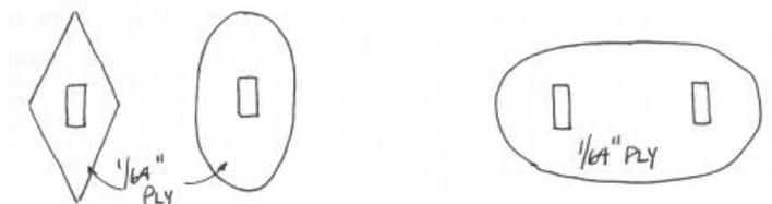
load. The load goes from the strips to the 1/64" ply and is transmitted across a larger surface of the foam board, tying them together, distributing the load.
