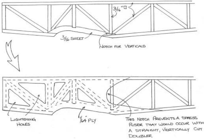
Many kits use a very poor design for fuselage construction.
