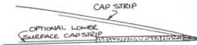
For light wings this works well. When dealing with cap strips, make sure the ribs are cut back so that the caps fair in with the spruce trailing edge.
