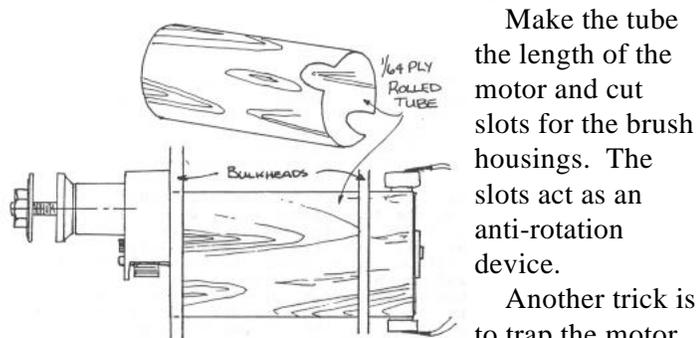
Another trick is to trap the motor with the gearbox. The motor can't move back and forth. Without the gear box, a snug fit is achieved by putting a strip of masking tape on the motor and pushing it into the motor mount for a snug friction fit.
