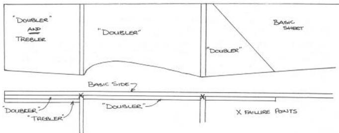
With the above construction, the plane comes in, bounces and breaks. There you have it - a fishhead, lying on the flying field.
