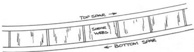
The bottom spar is under tension while the top spar is under compression. All of the materials, typically used for models, balsa, spruce, carbon fibre, are usually 3 to 10 times stronger in tension than in compression. If you want to build a strong wing, you have to think about the materials. Many designers put just a spar on the bottom. That doesn't make sense; it should be on the top. One of the worst airfoils is:
