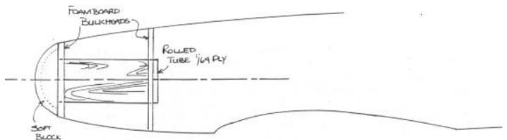
any more than that. Remember to tie the battery pack, the motor, the spar and the landing gear together. With foamboard half shell fuselages, on every bulkhead, somewhere in the middle, like with the crutch, set up a place where there is going to be a pair of lengthwise 1/8" x 3/8" pieces of spruce. This goes back and becomes the stabilizer seat and also ties into the motor tube.
