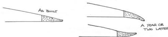
I haven't got the best solution, but what I've always done, because there isn't much strength required to hold the back of the wing straight, is to use a piece of sheet balsa, 1 1/2" wide and then, right at the back, glue on a piece of 1/8" x 1/4" spruce which I carve or sand to shape.
