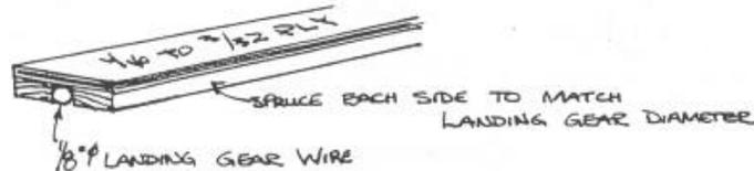
At the other end is where all the forces are going to concentrate. When you come in for a landing, the wire flexes back. The vertical block is trying to rotate out the front of the wing. If you are going to use maple anywhere, use it there.
