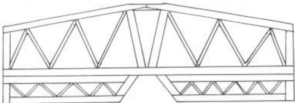
If you're worried about having the lumps showing through the covering, you can use a combination of these two. Put in the needed ribs and put in 1/8" x 1/16" diagonals that don't touch the covering.
