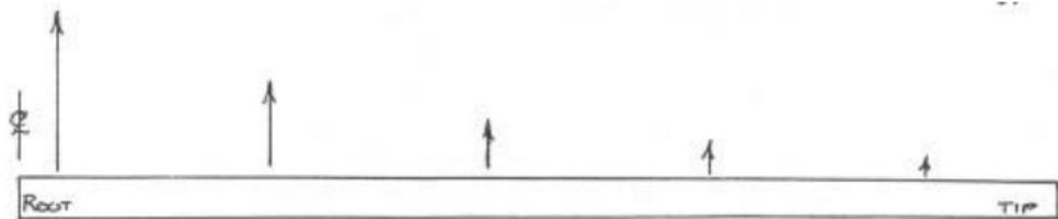
If you think about the load on the wing, the spar doesn't need to be as strong at the tip as at the center. Tapering the spar is a pain and it doesn't save much weight. If you have an extremely strong wing and want to use a "D" tube and cap strips, scarf in spar doublers for 2 or 3
