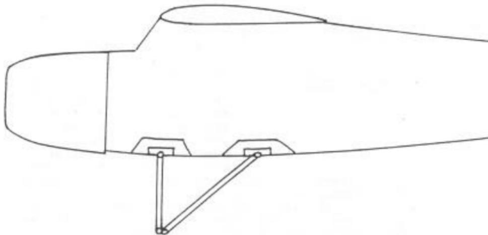
Like the trunnion block gear, this type also flexes out. Smaller diameter wire can be used than with the torsion bar landing gear of the wing. Use 1/8", 5/32", or 3/16" (for big planes), in wing torsion bar gear while 3/32" or 1/8" will work with this type of fuselage gear.
