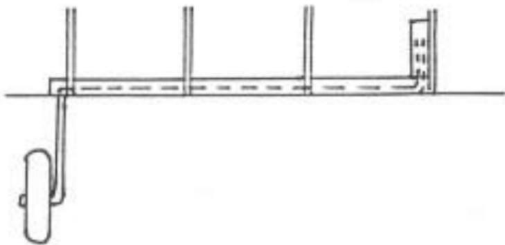
support it, the wire and the wheel. You want to make it into a retract. You've still got the wheel, most of the wire, some ply facing on the ribs to distribute load. You don't have those two pieces of torsion block on a retract, instead you've got the retract unit. These are pretty light. You've got a servo in the middle to run the retracts and you've got a slight difference of weight in the retracts themselves. To give you an example, the retracts on my 40 size Spitfire cost me 3.5 ounces.
