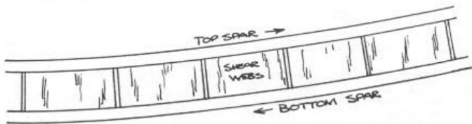
The bottom spar is under tension while the top spar is under compression. All of the materials, typically used for models, balsa, spruce, carbon fibre, are usually 3 to 10 times stronger in tension than in compression. If you want to build a strong wing, you have to think about the materials. Many designers put just a spar on the bottom. That doesn't make sense; it should be on the top. One of the worst airfoils is:
