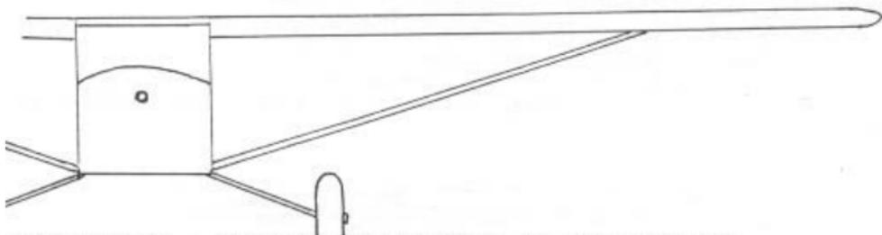
This creates a triangle and the strut is under tension.
