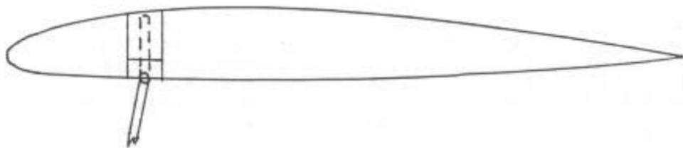
If you want to do a trunnion block set up use 1/32" ply laminated to the rib and notched to the spars. The
