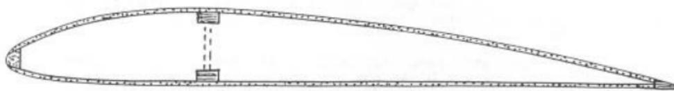
The front "D" tube is OK for up to 70 to 80 mph airplanes. When the planes start getting faster than that, or doing heavy duty aerobatics with lots of snap rolls, the secondary spar is a good idea. After that, you go to
