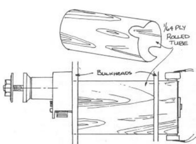
Make the tube the length of the motor and cut slots for the brush housings. The slots act as an anti-rotation device.
