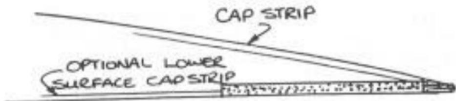
For light wings this works well. When dealing with cap strips, make sure the ribs are cut back so that the caps fair in with the spruce trailing edge.
