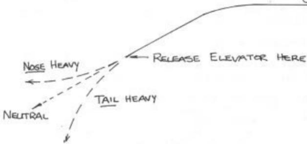
If the stick is released, and the airplane tries to do a half loop, the airplane is very **NOSE HEAVY**. When the airplane picks up speed, the negative incidence, (or slight up elevator trim), acts like up elevator and will try to make the plane loop. (The increased speed makes the trim have more effect.) As the CG is moved back, there is less of a downward load on the tail, so speed has little or no effect.
