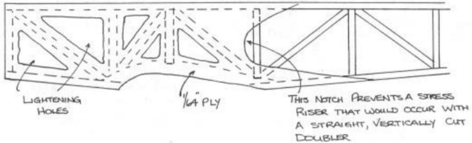
Many kits use a very poor design for fuselage construction.
