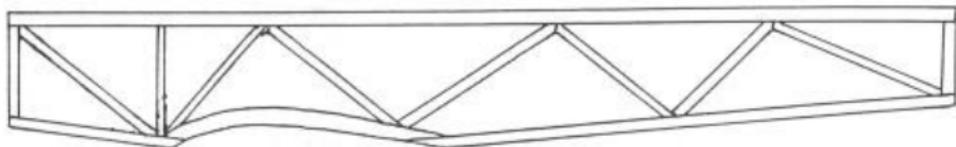
Even with verticals at the bulkhead position, you want to add a little strength so put in a diagonal like this:
