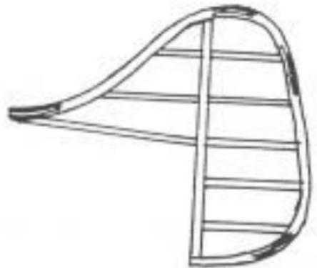
laminations, wrap it around the ply or foamboard form and tape it in place. Let it dry, take the tape off, pin it down and fill in inner structures. You can use 1/32" strip for the really small airplanes. It is very strong, like eggs and circles. It weighs virtually nothing.
