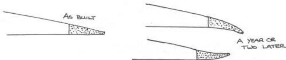
I haven't got the best solution, but what I've always done, because there isn't much strength required to hold the back of the wing straight, is to use a piece of sheet balsa, 1 1/2" wide and then, right at the back, glue on a piece of 1/8" x 1/4" spruce which I carve or sand to shape.
