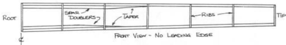
rib bays out. Taper the end to transfer the strength gently to the outer spar material at the tip. It only has to be 2 or 3 rib bays. The center section will be a little bit stronger, especially around the landing gear. That is where a lot of load is provided from landing. On most of my big airplanes and pattern airplanes, this is the spar system I use. If the upper and lower spars are 1/8" x
