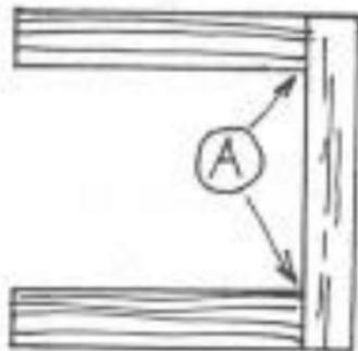
glue is not very strong in shear. There is not a lot of gluing surface. A good shear web in-between the spars is stronger, because the joint at "B" is not in shear and the glue is just there to hold it in place - not really much load on it.
