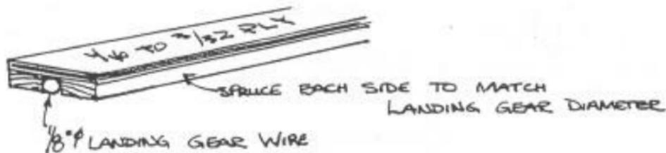
At the other end is where all the forces are going to concentrate. When you come in for a landing, the wire flexes back. The vertical block is trying to rotate out the front of the wing. If you are going to use maple anywhere, use it there.
