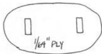
load. The load goes from the strips to the 1/64" ply and is transmitted across a larger surface of the foam board, tying them together, distributing the load.
