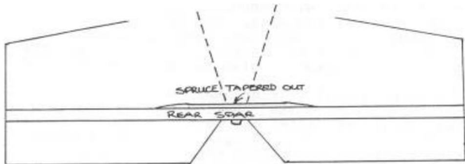
the fin down through the fuselage. Reinforce this with a small piece of spruce, tapered to avoid a stress riser.
