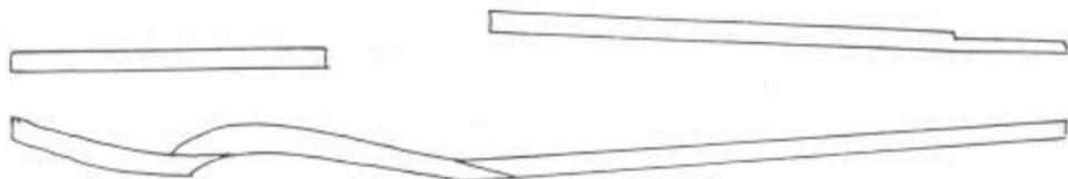
Make all bulkheads in two pieces and glue the bulkheads to the keel. Then add the stringers.
