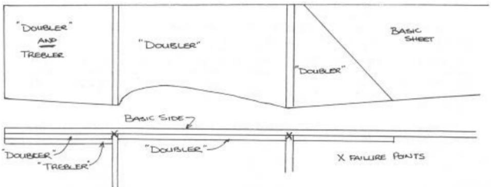
With the above construction, the plane comes in, bounces and breaks. There you have it - a fishead, lying on the flying field.
