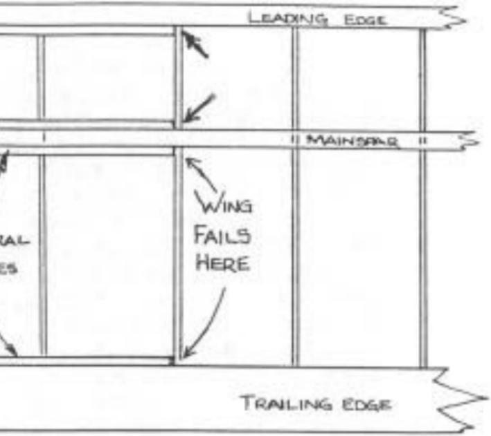
shear webs BETWEEN the spars. An "I" beam is much, much stronger. If you think about a wing, as the tip flexes up, the two spars appear to slide in opposite directions. The shear webs prevent this.
