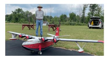
It is not my only float plane. My Martin MARS has a 120" wingspan and weighs 27 pounds. It uses Leopard motors and 4S 2000mAh LiPos.
