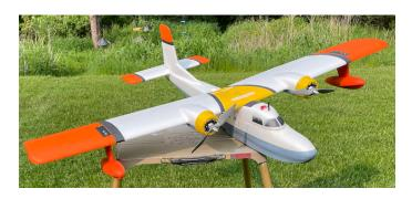
I am using Badass motors, Badass ESCs, APC 8x6 props (normal on left and pusher on right) and a 3S 2200mAh LiPo.
