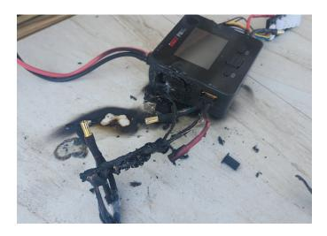
Then I realized the charger had melted down. One battery is fine. The other one has a good voltage of 25V but the balance tap is welded to the chargers balance board. It may be salvageable with a replacement balance plug if the insulation in the leads isn't compromised.
